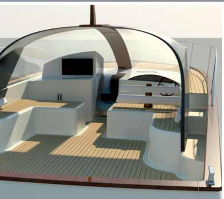
with its canoe-style bow. Although the deckhouse is open at the back for better natural ventilation, some sort of thermal resistant glass would probably be required to prevent the interior temperature becoming uncomfortably hot.
